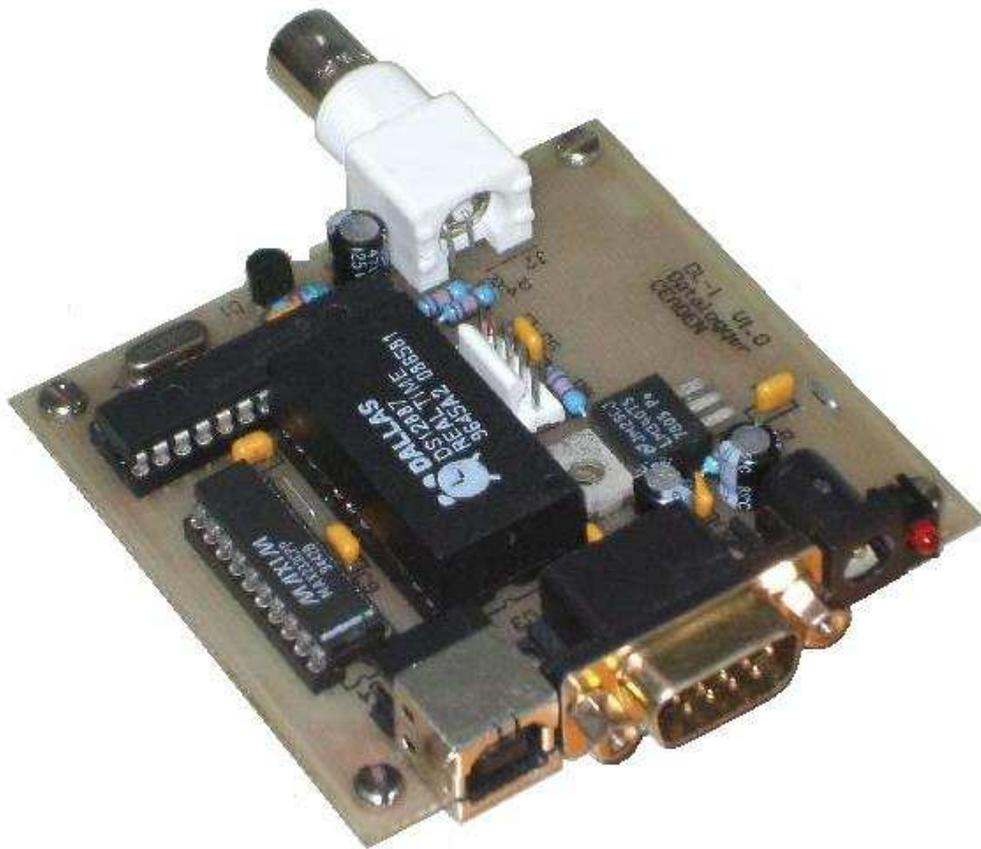
Figura 1. Datalogger's assembled board.
